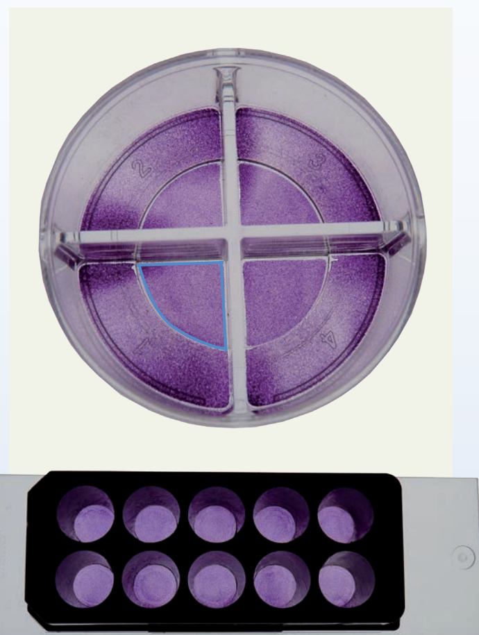
Figure 4: Crystal violet staining of a CELLview™ Dish and CELLview™ Slide verifying uniform cell distribution in the optical relevant areas.
